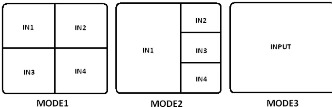
**MODE1:** The quad multi-viewer divides the four HD input to the same size and display on one screen. And now switch the input button on front panel or IR remote, the HDMI output audio will correspond to the selected input source.
