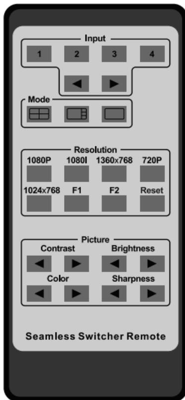
1. **Input select button:** press these buttons, the quad multi-viewer will select the corresponding input source, the front panel LED will indicate the selected input source status.
